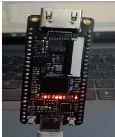
Figure 6: Tang Nano 9K development board used for SIMON32/64
